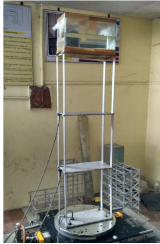
Figure 3. Tuned Liquid Damper
